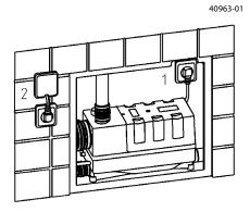
The electrical connection can be made in two ways: inside (1) or outside (2) the installation area.
