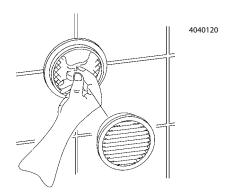
To change the active carbon filter in the unit venting system, only the push-fit venting grille has to be removed.
