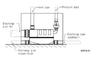
The assembly is placed into the installation space through the assembly opening and flexibly connected to the supply pipes by means of the sleeves and clamps.
