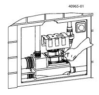
The motor/pump unit can be easily removed as a compact assembly. The tank remains in place.
