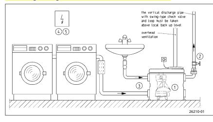
When used downstream of the backpressure level, German / European standard DIN EN 12056 requires the pressure pipe to be connected elastically and to be passed over the locally defined backpressure level in a loop. Moreover, the installation of a non-return valve is prescribed, which has been tested in keeping with German / European standard DIN EN 12050-4. In addition, we recommend an alarm system for monitoring.
