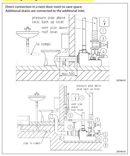
All types have DN 80 / PN 10 connecting flange, however with pipe socket DN 100. For this reason, non-return valves and shut-off valves need to be chosen for DN 80 only in case of direct erection. The downstream pressure pipe is connected to DN 100 by an elastic connection.
