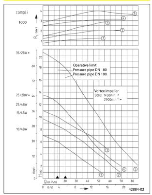
We reserve the right to change specifications without notice Pump performance is subject to ISO 9906 tolerances The minimum flow velocity in the pressure piping must be 0.7 m/s according to EN 12056. This data is represented in the performance curve as a limit of application.
