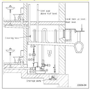
All types have DN 80 / PN 10 connecting flange, however with pipe socket DN 100. For this reason, non-return valves and shut-off valves for the pressure pipe need to be chosen for DN 80 only in case of direct erection. The downstream pressure pipe is connected to DN 100 by an elastic connection.
